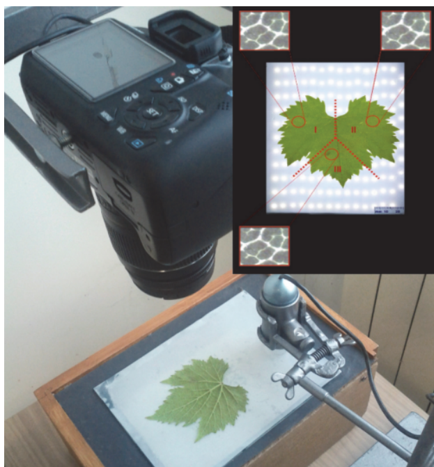
Fig. 1. Image acquisition set-up and crop (1 mm 2 ) image collection method. Leaf LED device (L × W × H: 12 × 7.5 × 5 cm) was equipped with 180 LEDs (SMD chip Samsung 5630; 6,000 K, thickness 2.4 mm). It was created to increase the sharpness of the data achieved and to highlight accurately the profiles of vein texture.
