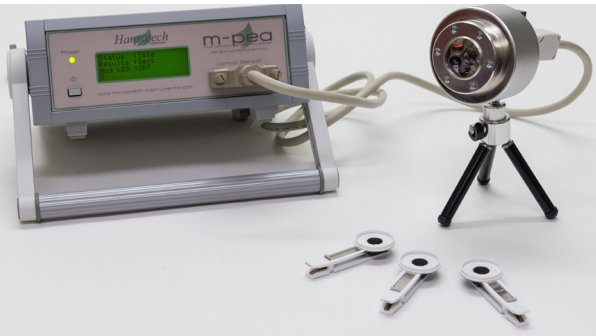
Fig. 9. The M-PEA ( Multi-Function Plant Efficiency Analyser ) developed by Hansatech Instruments Limited in cooperation with Prof. Reto Strasser and Prof. Vasilij Goltsev (Courtesy of Hansatech Instruments Limited, UK ).
