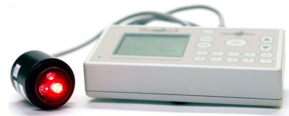
Fig. 8. Handy PEA consists of a compact, lightweight control unit encapsulating sophisticated electronics. This provides the high time-resolution which is essential in performing measurements of fast chlorophyll a fluorescence induction kinetics (Courtesy of Hansatech Instruments Limited, UK ).
